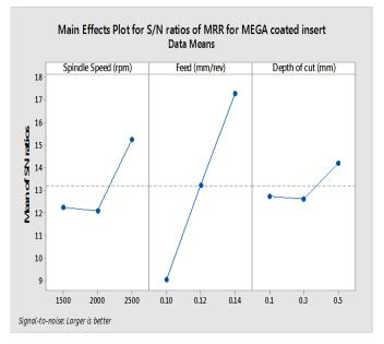
Figure no. 05 Main effects plot for S/N ratio of MRR using MEGA coated insert
