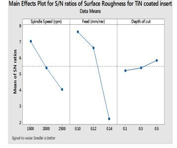
Figure no. 02 Main effects plot for S/N ratio of Ra using TiN coated insert
