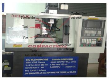
Figure no.01: Photographic view of experimental setup for machine
