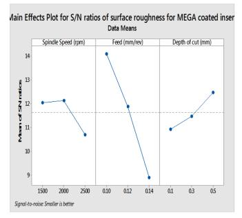
Figure no. 04 Main effects plot for S/N ratio of Ra using MEGA coated insert
