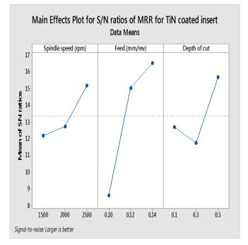
Figure no. 03 Main effects plot for S/N ratio of MRR using TiN coated insert
